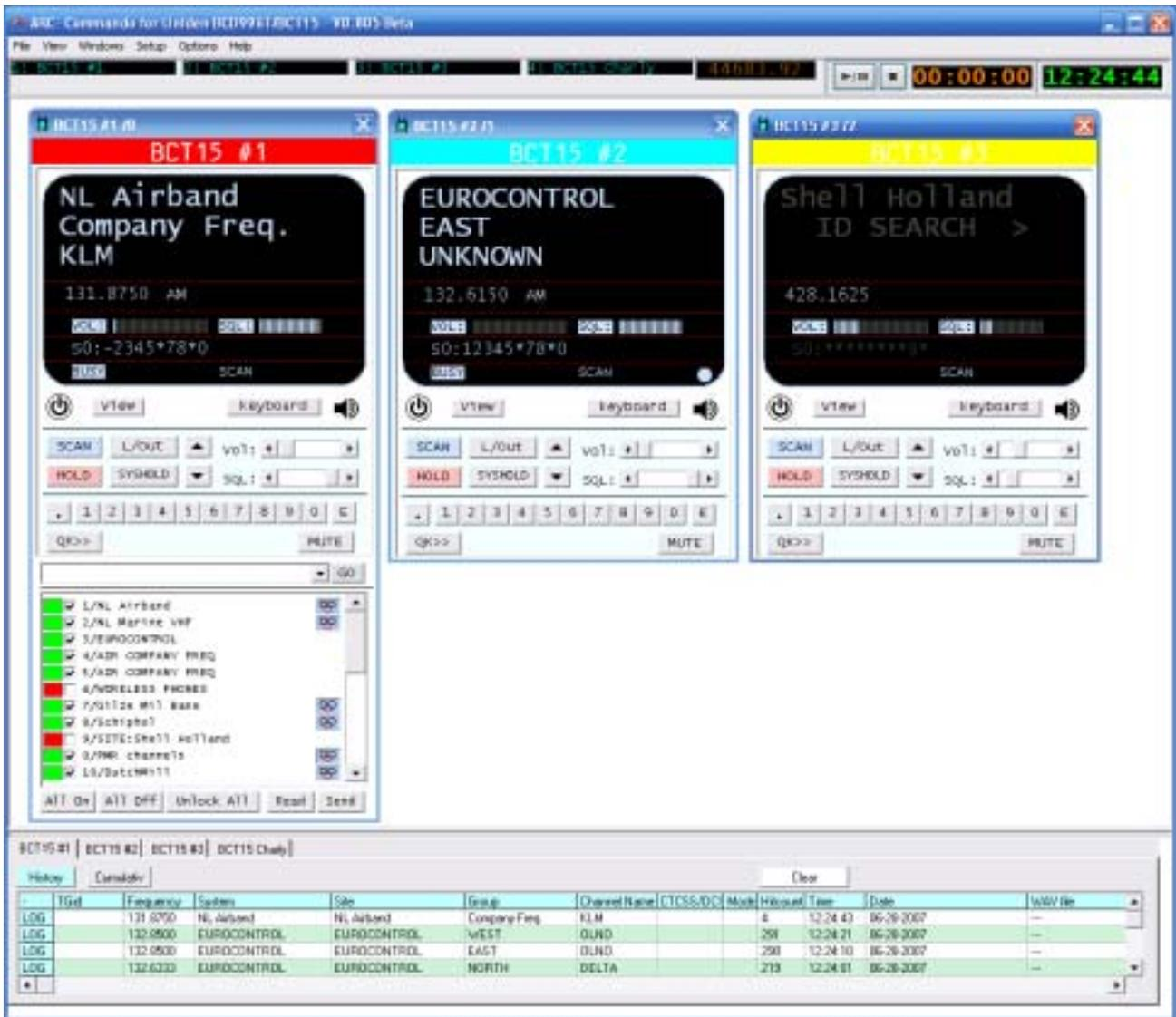
This screenshot shows three scanners, two scanners, BCT15 #1 and BCT15 #2, are 'active'. By using the VIEW button the window can be changed. Scanner #1 now shows the systems and a double click on the red/green button will enable FOCUS scan and disable all other systems.
