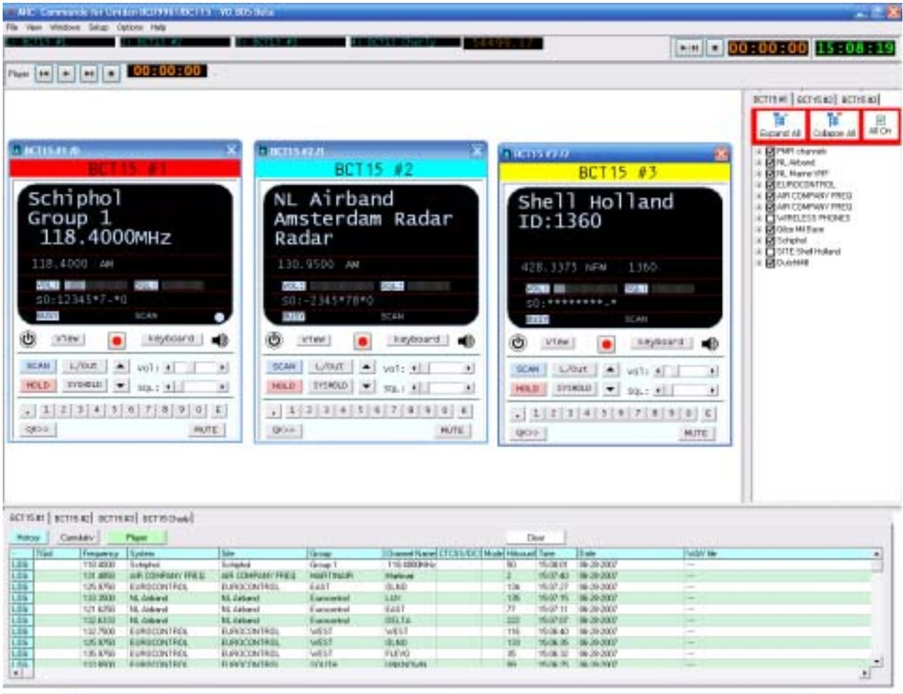
This screenshot shows three scanners, all 3 scanners active. Each scanner has a tab with a treeview for switching systems/groups on and off.
