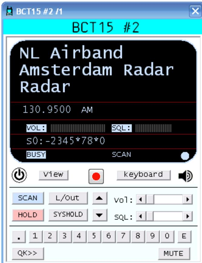
A three line display showing more information than is available on the scanner itself which only provides two lines. The software shows System, Group and Channel name. Additional information such as frequency, transmission mode and sub-audible tone is also shown.
