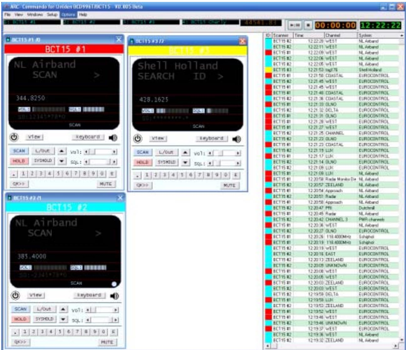
This screenshot shows three scanners and the multilog grid. For easy reference the colors that are assigned to the scanners are also used in the grid.
