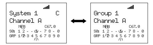
Even if the transmission ends, the scanner holds on the channel for the duration of the system delay time. After the system delay time elapses, if there is no transmission the scanner resumes scanning.
