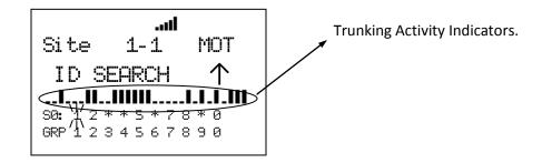
When the scanner receives a trunked system channel grant, the V-Ch blinks and the C-Ch lights. The scanner has 30 Channel Activity Indicators to visualize trunked system activity. This shows which site frequencies are in use.
