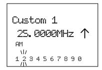
The scanner starts searching from the lowest frequency of the first turned on range and proceeds in ascending order. Or, it starts from the highest frequency of the last turned on range and searches in descending order. While searching, turn [Scroll Control] to change the search direction.
