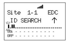
While the scanner is staying on a V-Ch, the voice channel blinks and its C-Ch turns on.
