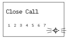
If the scanner has already received a Close Call hit and you press [Hold / 🍄], the scanner holds on the latest Close Call hit frequency. Or if it has not yet received a Close Call hit, the keypress is ignored and the scanner sounds an Error Tone.
