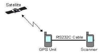
The formats of the GPS data that the scanner can receive are only GGA (Global Positioning System Fix Data) and RMC (Recommended Minimum Specific GNSS Data) based on "NMEA-0183 ver.3.01".
