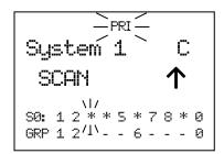
If there is no Priority Channel or all Priority Channels are locked out, the scanner displays "Priority Scan No Channel" and sounds an Error Tone. Then Priority Plus Scan stops.
